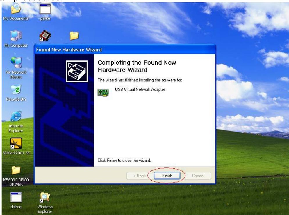
(xi) To check M5632 Super-Link whether install succeed, please go to the device manager to find the “USB Super Link Adapter” , and the installation is successful.
